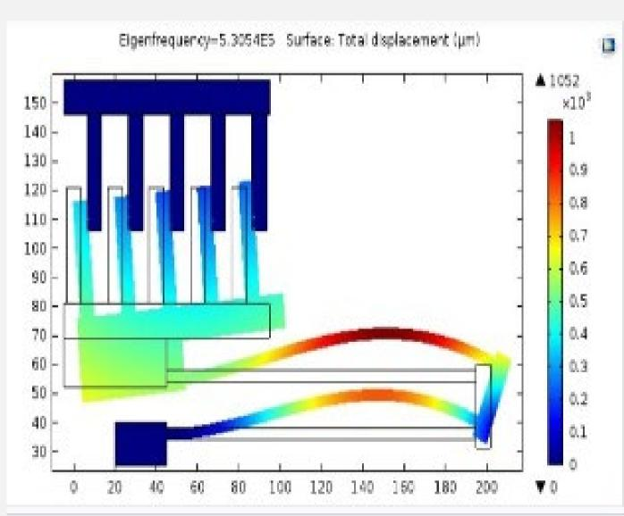
Stress distribution over different spring designs are simulated by COMSOL 5.0 a using a standard comb drive with increase in flexure length from 220µm to 280µm, displacement and capacitance increases from 1.063µm to 2.85µm and 327pf to 352pf respectively at 130V.
